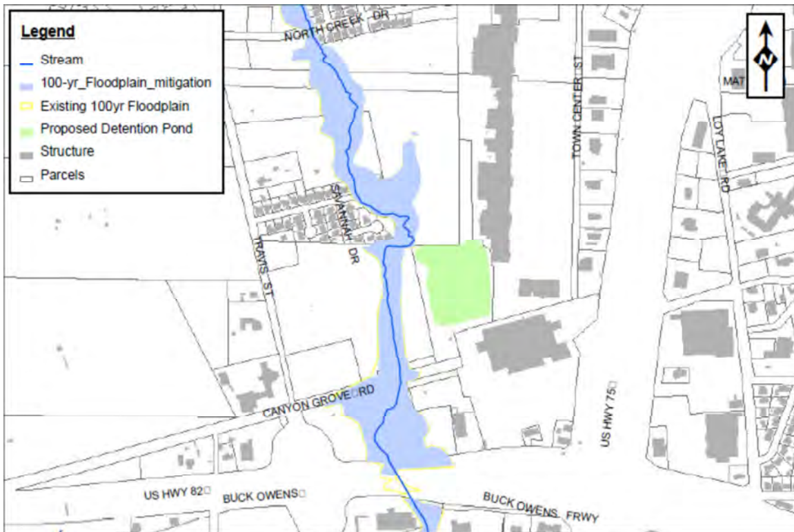
Figure 23. Town Center Detention Pond Modification. Project # 15.
